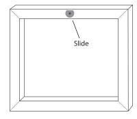
to hang your frame. Insert the Slide located on the top back of your frame, into the Bracket. The unique semi-circular Slide and grooved Bracket allow flexibility – so working with gravity, your frame will hang straight. That's Smart Level!
